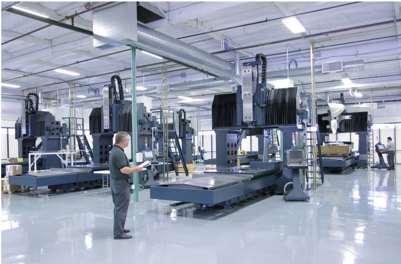
Tracy Peters checks out the installation of 5 of 8 Johnford custom 2600 F machines built to perform slow, super-high precision machining on large, critical lens components for the James Webb space telescope. The 8 machines were redesigned, rebuilt, tested and delivered in a total of 10 months by Taiwanese manufacturer Roundtop Machine Tool. "We considered that a remarkable performance," says Tracy Peters. Tinsley employs 102 people in a 150,000 sq ft facility.
